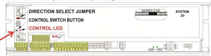
Pressing and holding the button causes the adjacent red Control LED to pulse "on" approximately once per second. The number of pulses determines the resulting effect:
